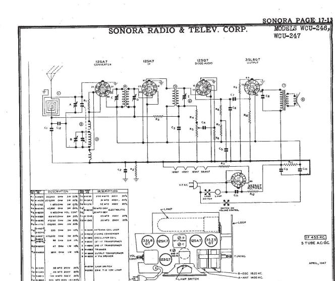
Lack of sensitivity and poor tone quality may be due to any one or a combination of causes such as weak or defective tubes or speaker, open or grounded bias resistor, bypass condenser, etc. Never attempt to realign set until all other possible sources of trouble have been first thoroughly investigated and definitely proved not to be the cause.
